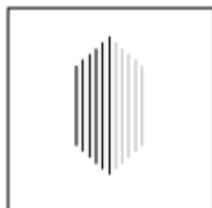
Figure 21.8. You cast a ray for each vertical column. If a wall is struck, you draw a line based on the distance the ray went.
