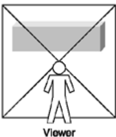
Figure 21.5. Ray casting presents an image of the world in a first-person perspective.
