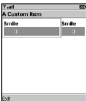
Figure 19.5. The first smiley item has the LAYOUT_EXPAND set, causing it to assume the majority of screen space (see FormLayoutExample).
