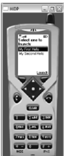
Figure 4.10. When loading a JAR containing multiple MIDlets the emulator will ask which one to execute.
