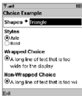
Figure 19.7. A demonstration MIDlet showing a drop-down style ChoiceGroupa list containing items using different fonts, as well as two choices using different fit policies
