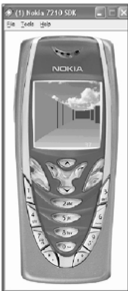
Figure 21.23. The left-hand wall shows the results of not detecting edges properly.
