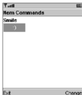
Figure 19.8. An example of an item command; note that the "change" command is only displayed when the smiley item is focused.
